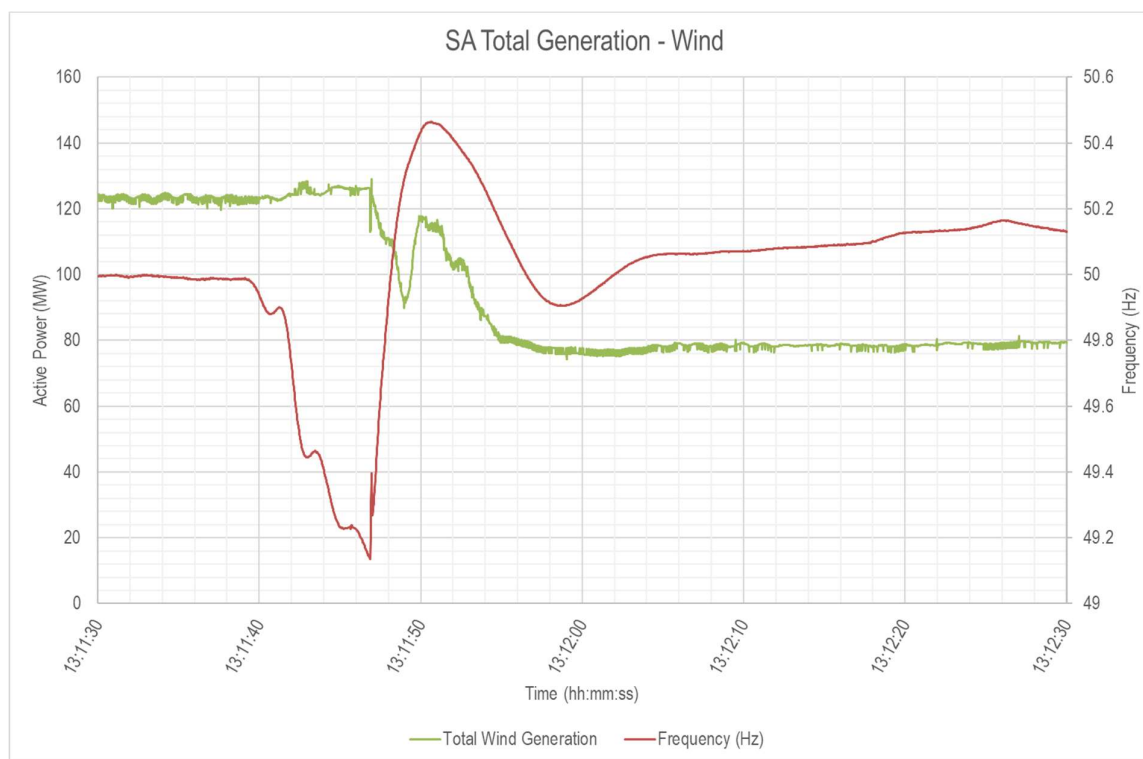
Figure 36 Aggregate SA transmission-connected wind generation response – short-term
