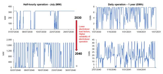
Figure 10: Half-hourly and daily operation of CQ hydrogen load in 2030 and 2040 from Plexos outputs
