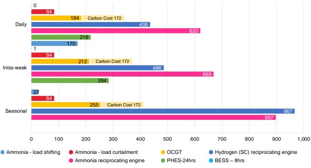
Figure 21: Levelised cost of different firming technologies by cycling interval (\$/MWh)
