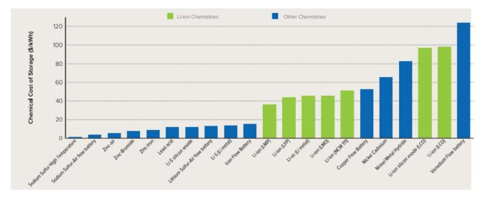
Figure 4 - Estimated Cost of Raw Materials for Different Battery Chemistries. Source: Tyson and Bloch (2019)
