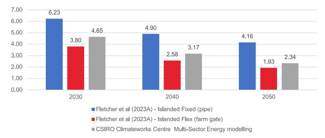
Figure 1 – Levelised cost of hydrogen (\$/kg H<sub>2</sub>) projections
