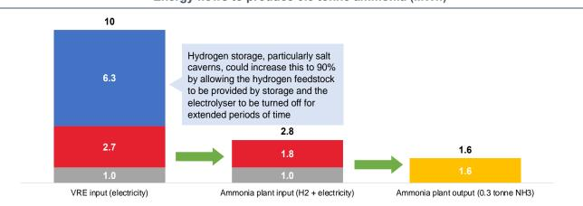
Green ammonia plant operating at minimum capacity (30% nameplate) Energy flows to produce 0.3 tonne ammonia (MWh)
