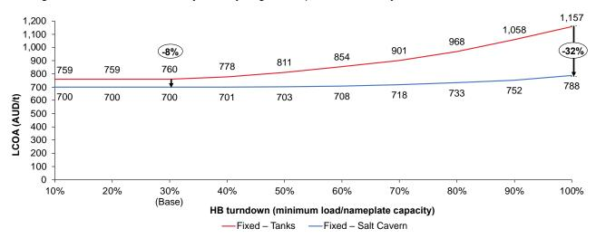
Figure 23: LCOA at different ammonia plant turndowns (Barcaldine 2040). Source: Fletcher et al (2023B)
