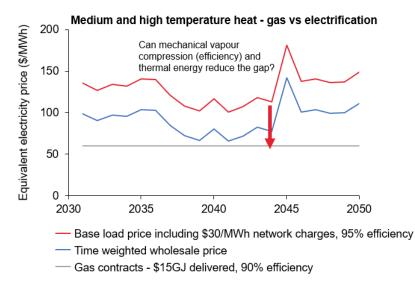
Figure 22: medium and high temperature heat - gas vs electrification
