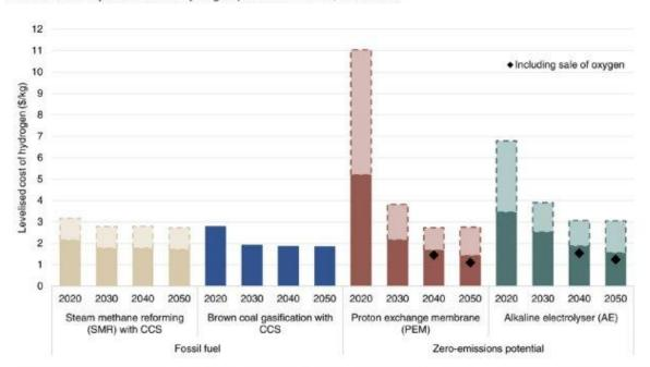
FIGURE 18: Projected costs of hydrogen production routes, 2020-205058
