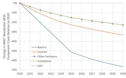
Figure 6 - Changes in projected component costs for residential BESS. Source – NREL (2024A) - BNEF. "Energy Storage System Costs Survey 2019." BloombergNEF, October 14, 2019.
