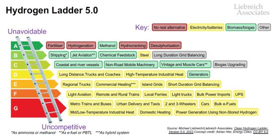
Figure 19: Hydrogen Ladder 5.0. Source: Liebreich Associates (2023)
