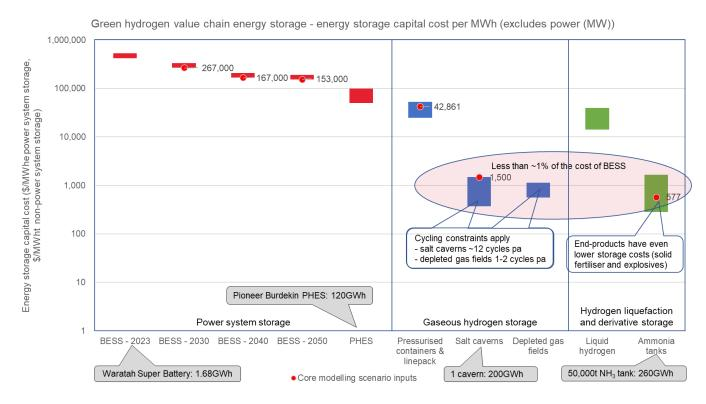
Figure 26: Energy storage capital cost per MWh (excluding power (MW)) in green hydrogen and ammonia value chain
