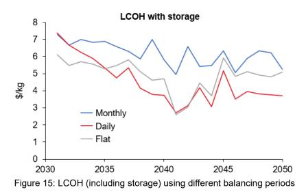
Daily balancing results in slightly more utility scale BESS and gas (Figure 16) an a largely unchanged total system cost (Figure 17). This analysis highlights that changing from monthly balancing to daily balancing had limited impact on the ISP model while delivering a more reasonable LCOH outcome. In contrast, a flat hydrogen load requires significantly more BESS and results in a much higher system cost.
